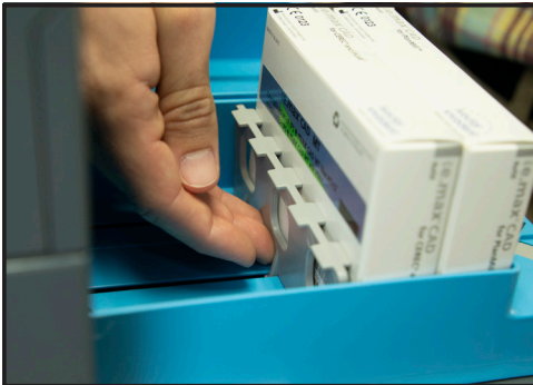
5) Pull gray slide tight against the back of block packaging, push base forward to lock in place.
